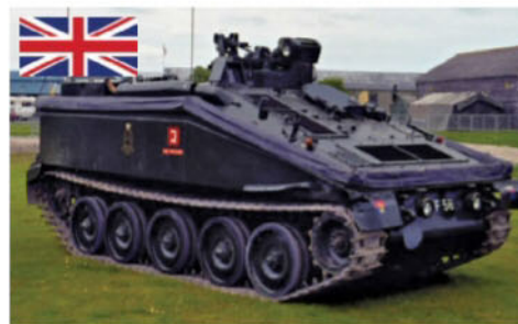
This British tank destroyer was introduced in 1975 and saw service in the Gulf War. Its Swingfire missiles have a range of 4,000m (13,120ft)
